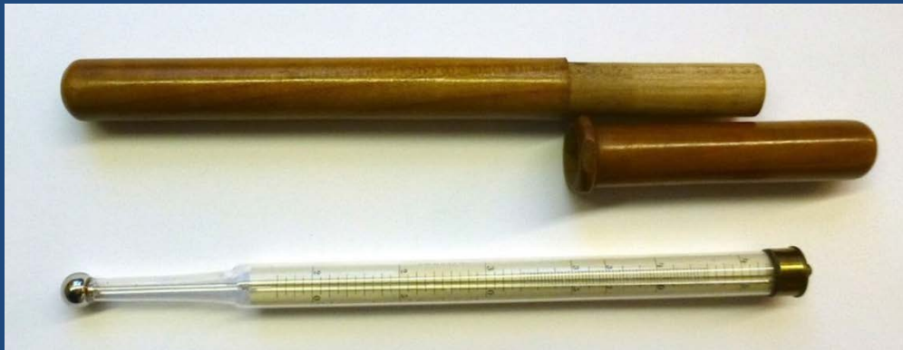
A Wunderlich thermometer, 10 inches long, with wooden case. Axillary temperatures took 30 minutes. Photo courtesy of medhxtour.
